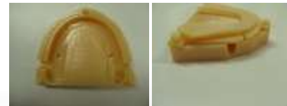
Printable molds allow for accurate acrylic placement
